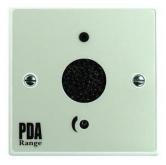
Typically, up to 10 Outreach plates (any mix) can be daisy-chained to one balanced line level connection with cable lengths up to 100m easily achievable using standard two-pair audio cable (i.e. belden 8723). Each plate requires four wires; two balanced line (Line/A+,Line/A -), one ground(GND) and one power connection (V+= 12-32V d.c.).
